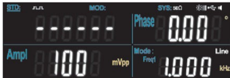
Picture 4-20 Set frequency sweep waveform
